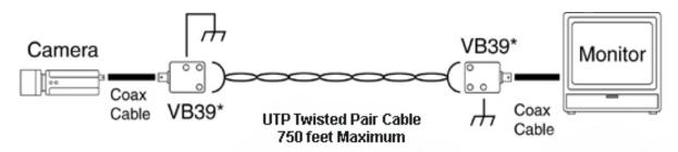
In the diagram shown above, two VB39M devices are used; one at the Head-End (monitor location) and the second at the camera location. No voltage is required for the baluns, since they are passive devices. Video is sent back to the monitor over the UTP cable by means of the two baluns operating as video transceivers. Note the Earth Ground connections for the surge protection circuits.
