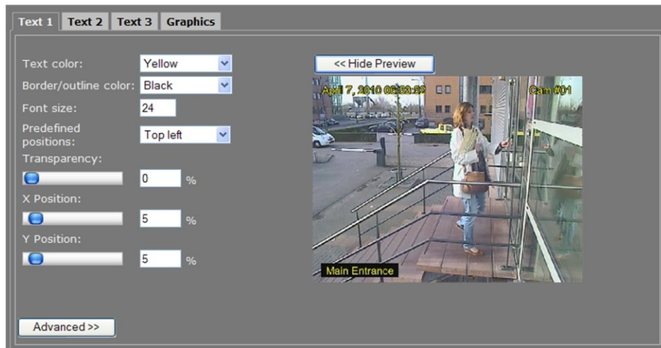
Text 1 tab with 3 OSD bars in the preview. Render modes: 'Outline' (top left & right) and 'Border' (bottom left).
