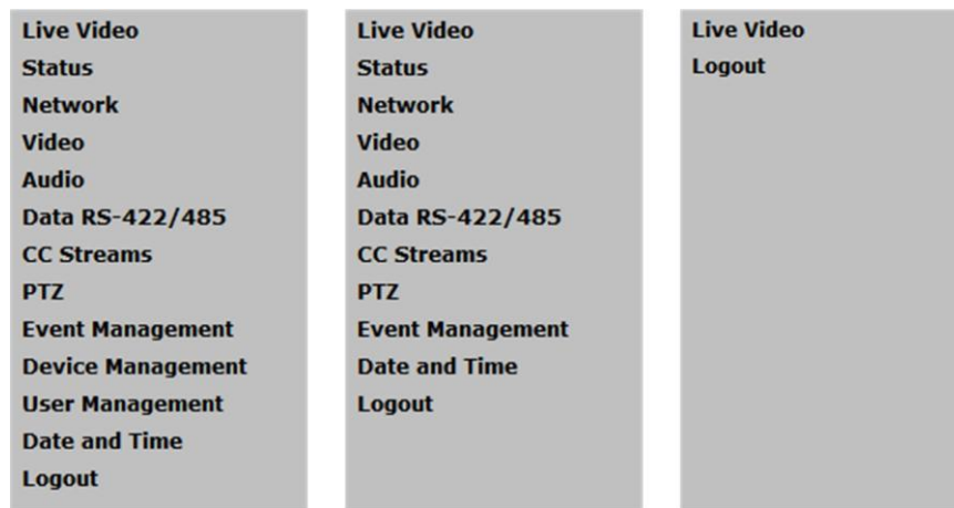
BC620WDR menu options available to (from left to right) Admin, Operator, and Viewer accounts
