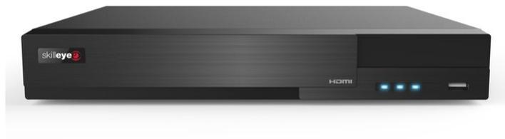
**DVR 5in1 960H/HD-TVI/AHD/HD-CVI/IP, 16 Ingressi più 2 IP (sino a 18), 12fps@1080pLite o 25fps/720p più 2 IP 5MP/25fps, HDMI/VGA/SPOT, Fanless, NDAA.**
