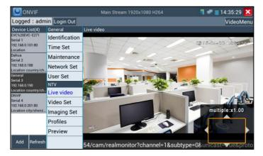
When the image is enlarged, if not operate on touch screen, it can operate by the keyboard ,press the key (TELE ) to zoom in , press the key (TELE ) to zoom out ,press upward and downward key to move
