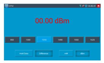
Data hold and Relative measuring use together, the data is yellow while the function is effect.
