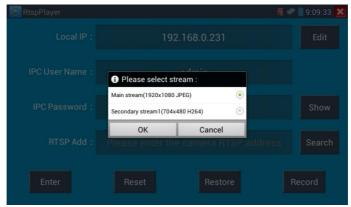
Note: in the event the ip tester does not auto detect the rtsp stream, refer to the specific camera manufacturer for the specific rtsp stream url. you may find this on line with a search of the camera model number and the word rtsp.
