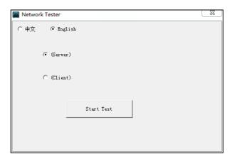
Tester as Client, tester's IP address is:192.168.0.230. The Server and the Client are at the same network segment, but with different IP address. Input Server's IP address 192.168.0.89 in the tester and click "Start" to test network bandwidth.
