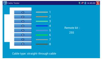
Test LAN cable or telephone cable.
