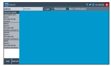
If your IP camera does not appear after scanning the network, you can manually add an IP camera by clicking on the "Add" button on the bottom left. The URL address should be identical to the ONVIF camera service address. (With your camera's IP address entered into the URL). Click OK to add the manually entered camera and then click the "Refresh" button.
