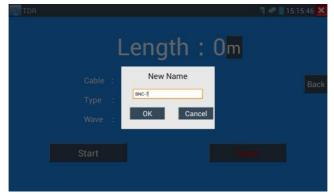
Application: TDR test is the use of pulse reflection method, to transmit pulse signal for tested cable, when cable is open circuit or short-circuit, reflected pulse is generated, the tester receives and deals with the reflected wave, measurement results displayed on the screen. TDR can test cable open circuit and short circuit, help engineer quickly find the cable's problem location. It is more convenient and efficient to repair the faulty cable.
