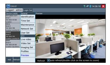
**Network setting**: Click "Network Set "to change the IP address settings. Note: Some cameras are not fully ONVIF compliant and cannot support changing their IP address, so there is no change after
