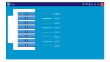
Connect a network cable from a PoE switch to the IP tester's PSE IN port. Connect an IP camera or other PoE using node to IP tester's LAN port, the PoE voltage and the cable's pin connection status show on the screen.
