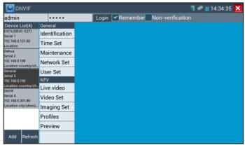
After selecting your ONVIF camera, enter the IP camera's username and password at the top left of the screen and then click "Login". After you log in, click on the camera under "Device List". Once you are connected to the camera, the following options become available: Identification, Time Set, Maintenance, Network Set, User Set, Live Video, Video Streaming, Image Set and Profiles.
