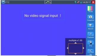
if not use touch screen to operate, press the key (TELE) to zoom out, press the key (XWIDE) to zoom in, press upward and downward key to move the image
