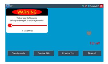
VFL four status can select—"Steady mode", "Evasive 1Hz", "Evasive 2Hz"and "Time off". Click button "Steady mode" to enter steady status, click button "Evasive 1Hz" and "Evasive 2Hz, to enter pulse mode, click button "Time off", VFL is turned off. Timed turn off can select (5 mins, 10 mins, 30 mins, 60 mins and 120 mins).
