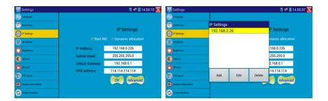
After setting an advanced IP address (refer to the photos above), the unit can test two network segments (192.168.0.0) and (192.168.1.0)
