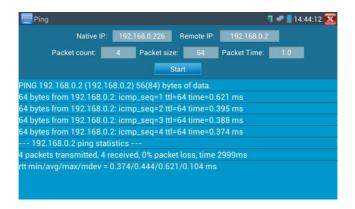
**Application:** PING testing is the most conventional network debugging tools. It is used for testing if the connected IP camera or other network equipment's Ethernet port is working normally and the IP address is correct.
