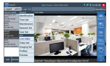
**ONVIF PTZ control:** Tap the image in the direction you want the PTZ camera to move. Tap the left side of the image to move left, right to go right, up to go up and down to go down. Compatible IP PTZ cameras will rotate accordingly. PTZ rotation direction is displayed on top left corner of the image.
