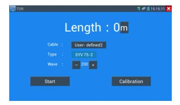
1.Select user-defined and click "Calibration "to enter test, click "user-defined 1" can define cable name, such as: AiPu BNC-5
