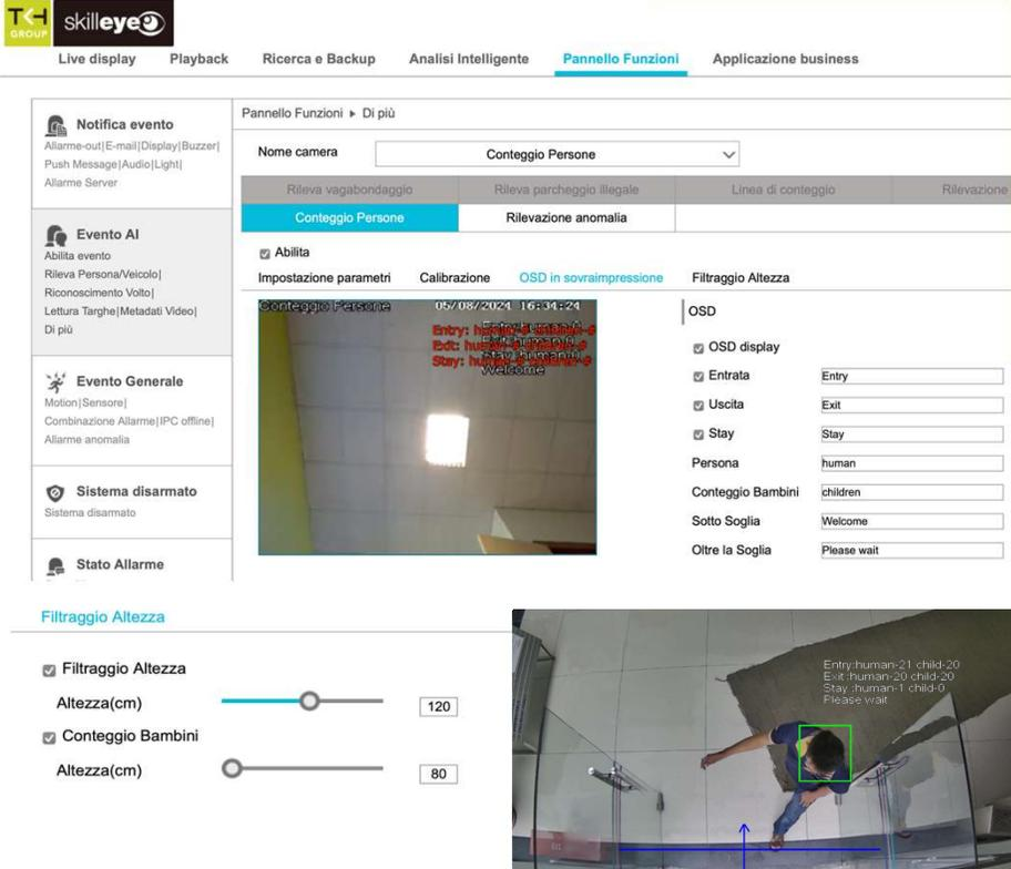
The screenshot shows the 'Pannello Funzioni' (Function Panel) for the 'Conteggio Persone' (Person Counting) camera. The interface includes a sidebar with navigation options like 'Notifica evento', 'Evento AI', 'Evento Generale', 'Sistema disarmato', and 'Stato Allarme'. The main area is divided into several sections:
